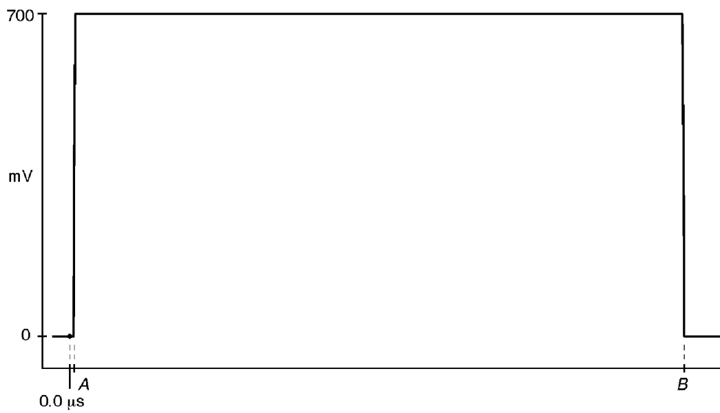
Figure 1-35: Active Picture Markers, Vertical Limits, Y Channel Only
